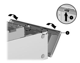
removing the front bezel from the 8000 series
